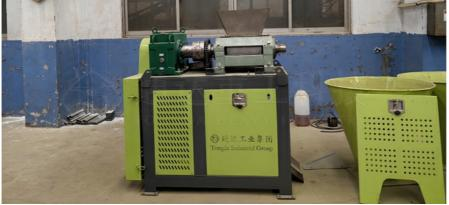
Working principle: adopts the design solution of extrusion sliding model, the raw materials pass through double roller. after that, enter into scattering room, come out as granulation, a sieving was mounted at the bottom of the machine, which is customized according to client's requirement, last, sieve out the granules which is qualified, the rest of materials return to mixer and be re-granulated.
