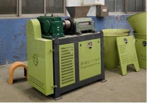
Working principle: adopts the design solution of extrusion sliding model, the raw materials pass through double roller, after that, enter into scattering room, come out as granulation, a sieving was mounted at the bottom of the machine, which is customized according to client's requirement, last, sieve out the granules which is qualified, the rest of materials return to mixer and be re-granulated.
