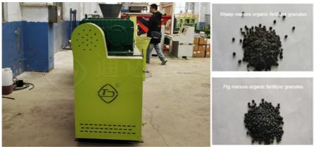
Working principle: adopts the design solution of extrusion sliding model, the raw materials pass through double roller, after that, enter into scattering room, come out as granulation, a sieving was mounted at the bottom of the machine, which is customized according to client's requirement, last, sieve out the granules which is qualified, the rest of materials return to mixer and be re-granulated.
